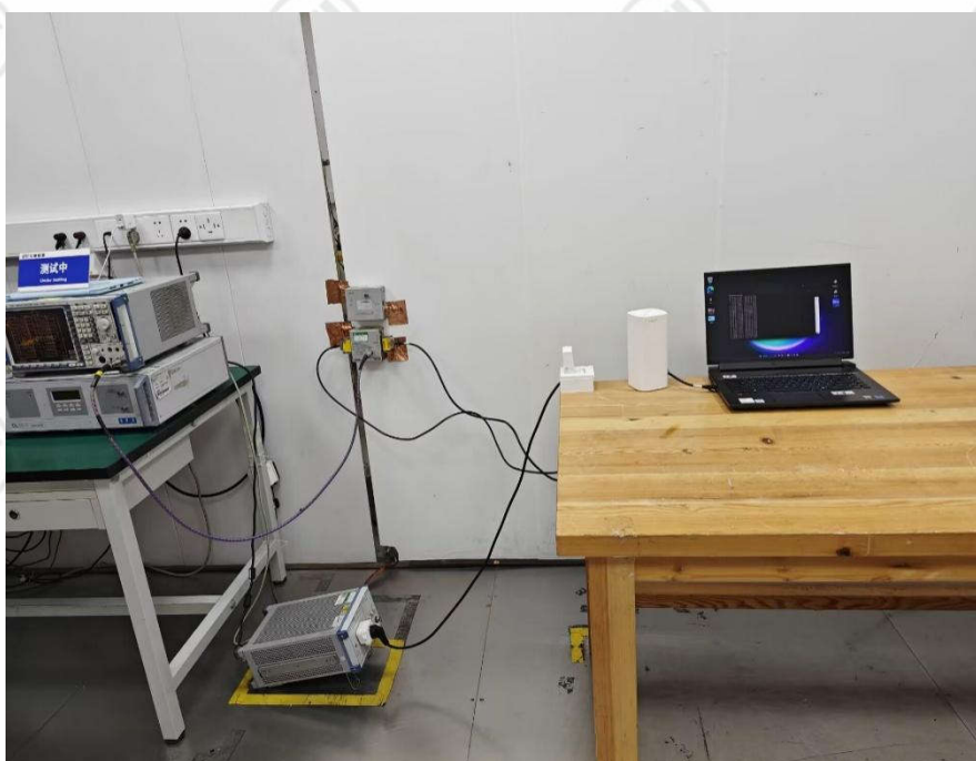
Conducted Emissions Test Setup-2
