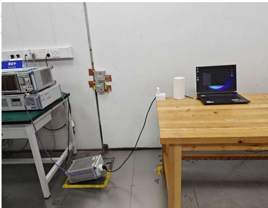
Conducted Emissions Test Setup-3
