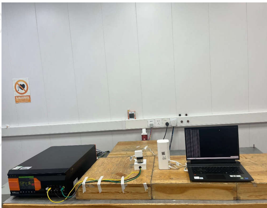
Electrical Fast Transients Burst Test Setup-2
