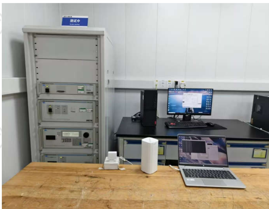
Voltage Dips And Interruptions Test Setup-1
