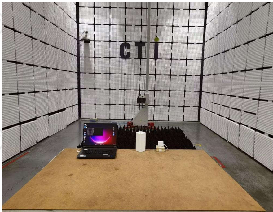
Radiated Emissions Test Setup-1
